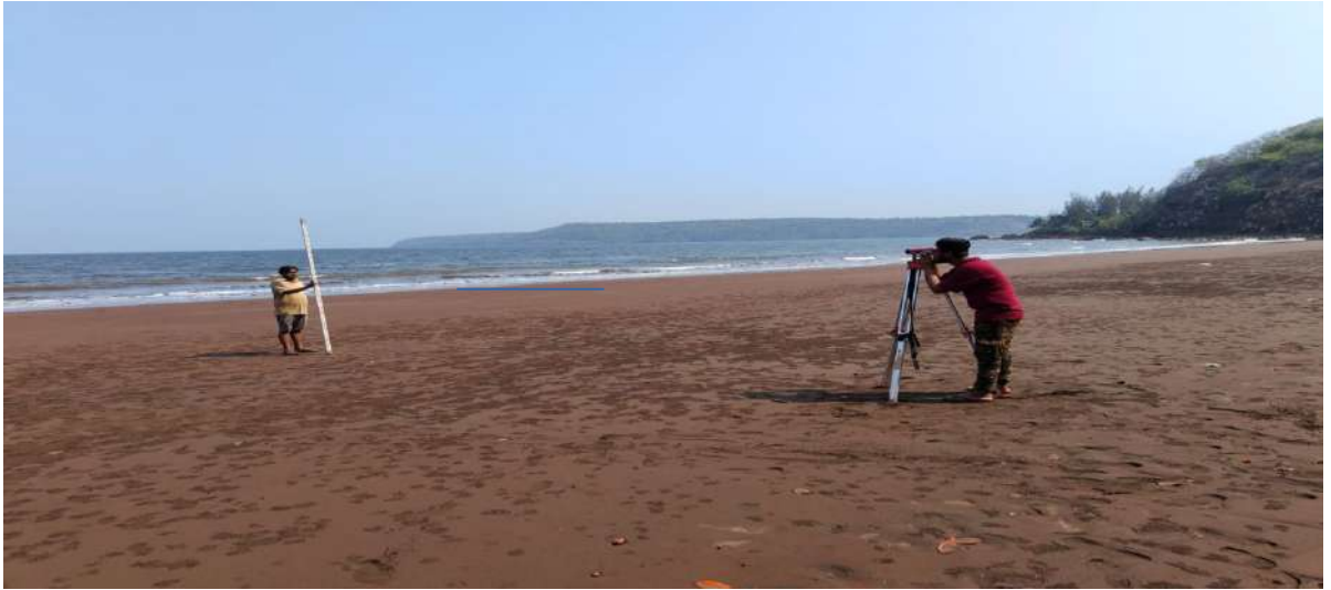
Beach profile using Dumpy level at Rohile beach
